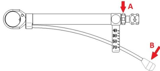
Apply pressure to the component at **arrow B**. The required torque is reached when the centre of the flexible rod is in line with the corresponding scale marking.
