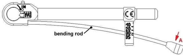
Apply pressure to component A in the direction of the arrow.
